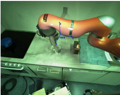
Fig. 3. Robot's camera view while grasping a cup. Objects are often partially occluded during grasping.
